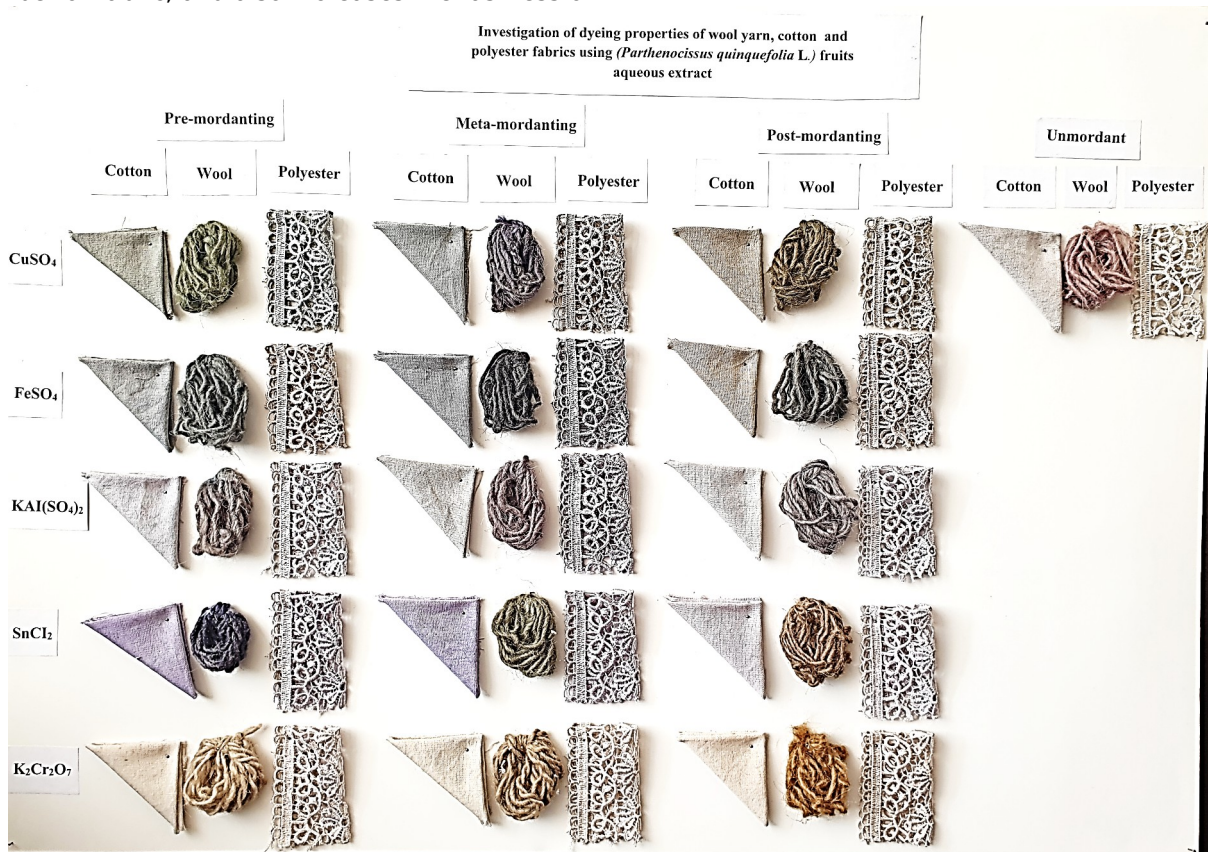
Figure 4: Samples of cotton, wool yarn and polyester fabric dyed with Parthenocissus quinquefolia L. fruit extract.
