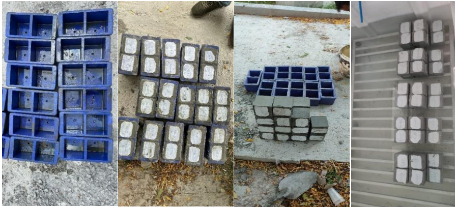
Fig. 2 Lubricating the molds, removing the samples and placing them in the curing pool
