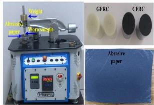
Figure 1. Wear device and GFRC/CFRC composite samples
