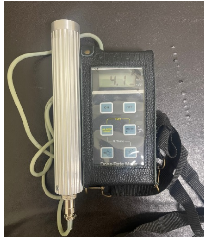
Figure 2. Geiger-Muller Detector, NEB.211B
