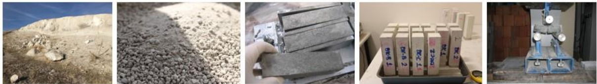
Figure. Sample production and test process with aggregates of different grain sizes.
