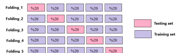
Figure 3. Using 5-fold cross-validation and data set splitting
