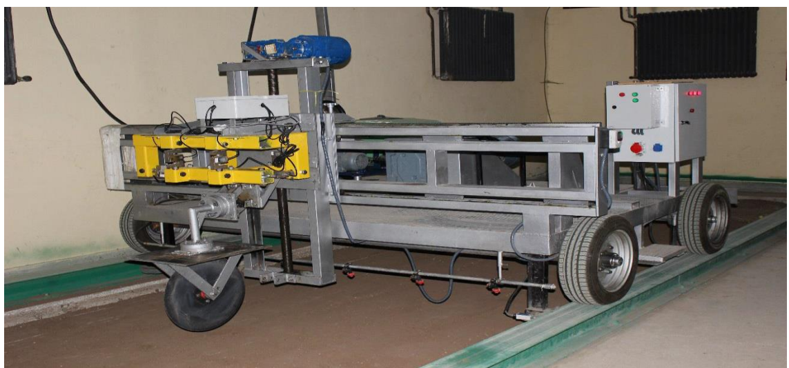
Figure 1. Soil bin carriage
