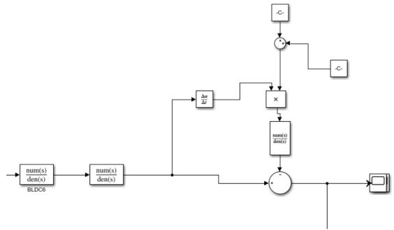
Figure 5. Simulink representation of stuck point model
