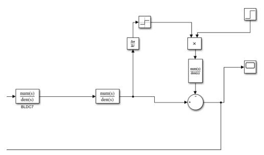
Figure 6. Simulink representation of moving friction point model
