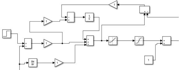
Figure 3. Clamping Anti-windup PID model in Simulink
