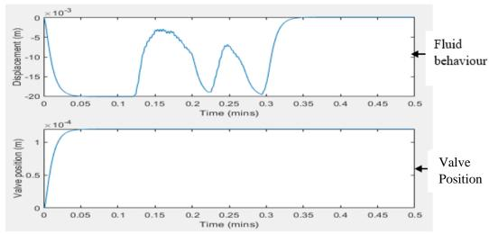
Figure 9. Response of valve at breakaway point
