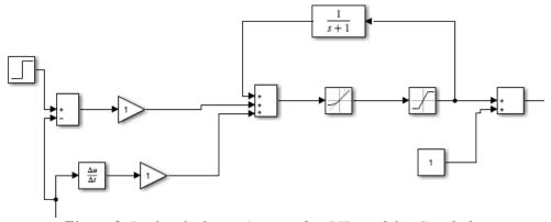
Figure 2. Back-calculation Anti-windup PID model in Simulink
