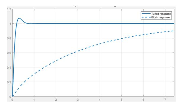
Figure 1. Anti-windup controllers' tuned response
