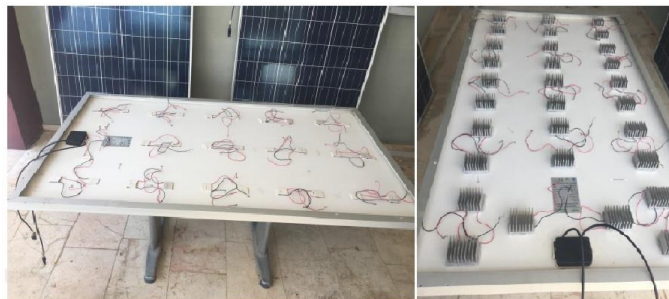
Fig.21. The installation of (a) thermoelectric generators (b) aluminum fins on the back surface [44]
