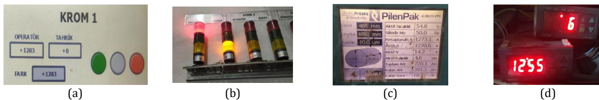
Figure 6. Chrome Plating Machine: a) HMI Screen, b) Alarm Lights, C) Machine Information and D) ENDA Current Visual.
