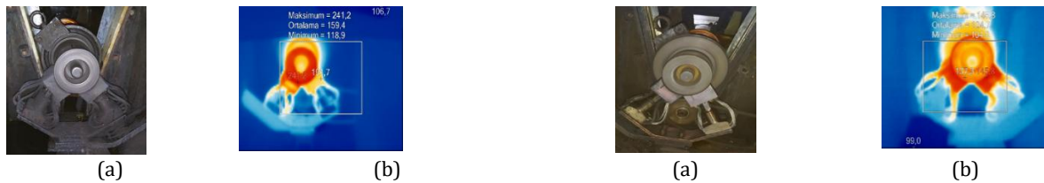
Figure 7. Chrome Plating Bath Error Status: a) Adapter, and b) Thermal Camera Images.
