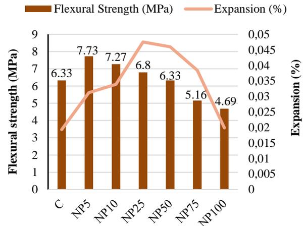
Figure 4. Relationship between flexural strength and expansion results
