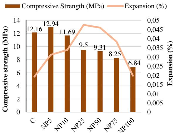
Figure 3. Compressive strengths-expansion results
