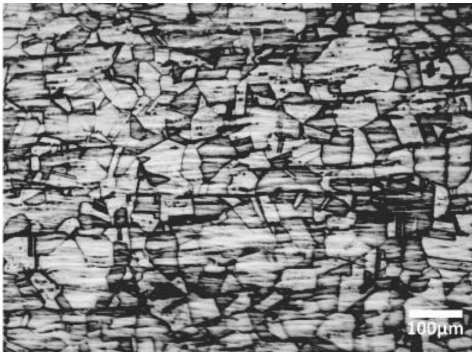
**Figure 1.** Microstructure of the as received austenitic stainless steel sample
