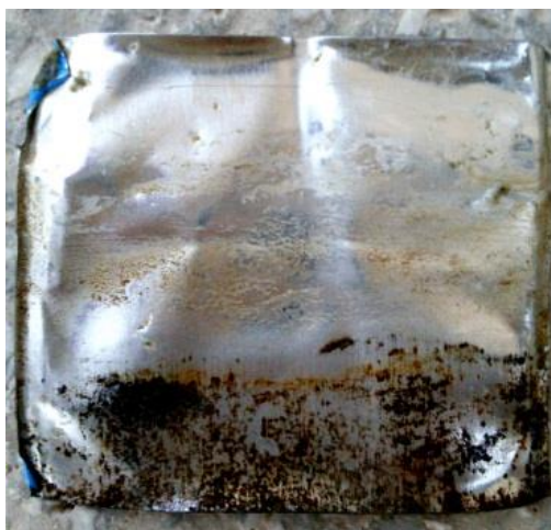
Figure 4. Corrosion of zinc anode of in this study
