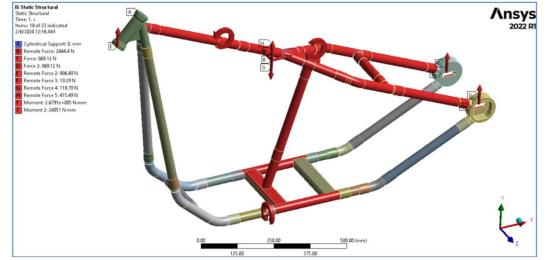
Figure 28. Boundary conditions for frame dynamic load analysis in cornering for Hybrid Frame
