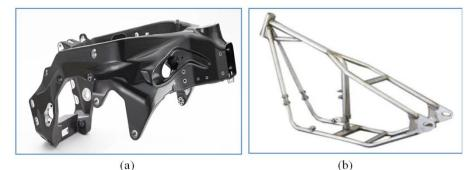
Figure 35. (a) Monoblock and (b) Tubular Motorcycle Chassis
