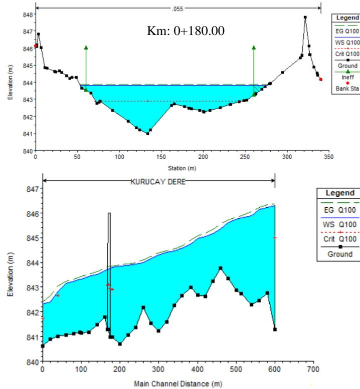
**Figure 4 (continued).** Km: 0+167.55 (upstream), 0+175.00 (bridge) and 0+180.00 (downstream) and water surface profiles of the entire channel.
