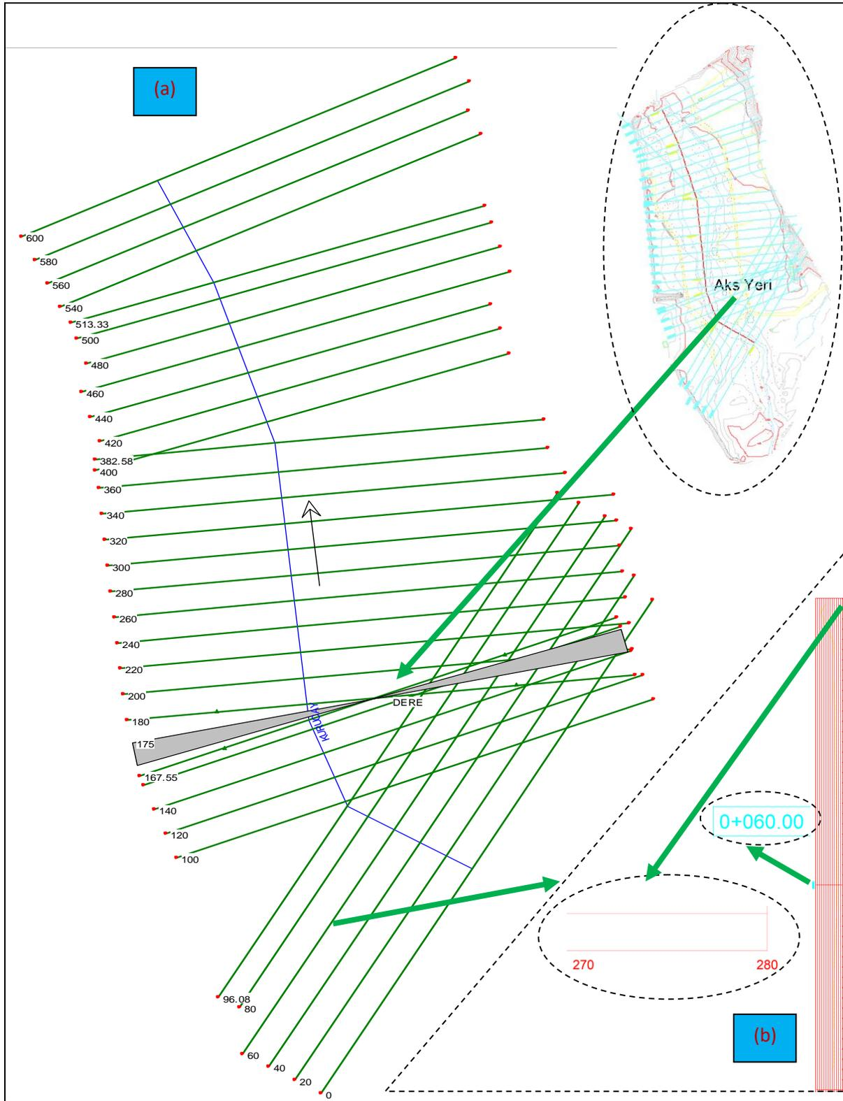
Figure 3. (a) Cross-sections from AutoCAD Civil 3D, (b) Detailed cross-section at Km 0+060.00.
