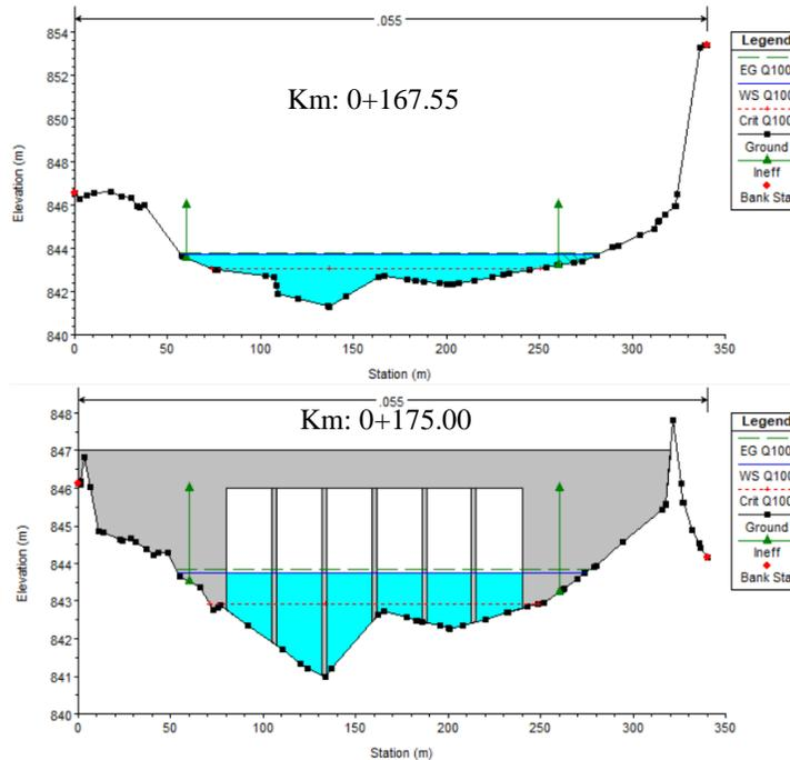
**Figure 4.** Km: 0+167.55 (upstream), 0+175.00 (bridge) and 0+180.00 (downstream) and water surface profiles of the entire channel.
