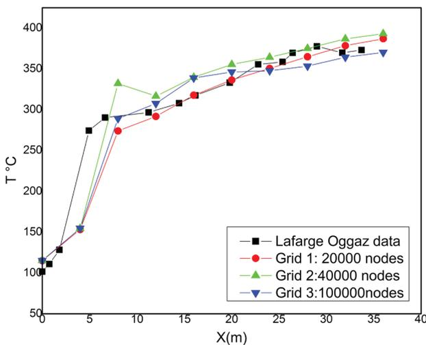
Figure 6. Mesh size effect on the temperature profiles.
