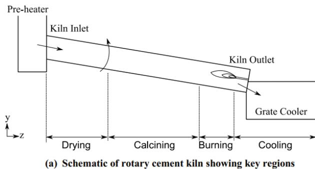
**Figure 1.** Figure 1. Schematic view of the rotary cement kiln [29]. Adapted from: Csernyei C, Christopher M. Numerical Modelling of a Rotary Cement Kiln with External Shell Cooling Fans. Electronic Thesis and Dissertation Repository. 2016. Available at: <https://ir.lib.uwo.ca/etd/3682>.
