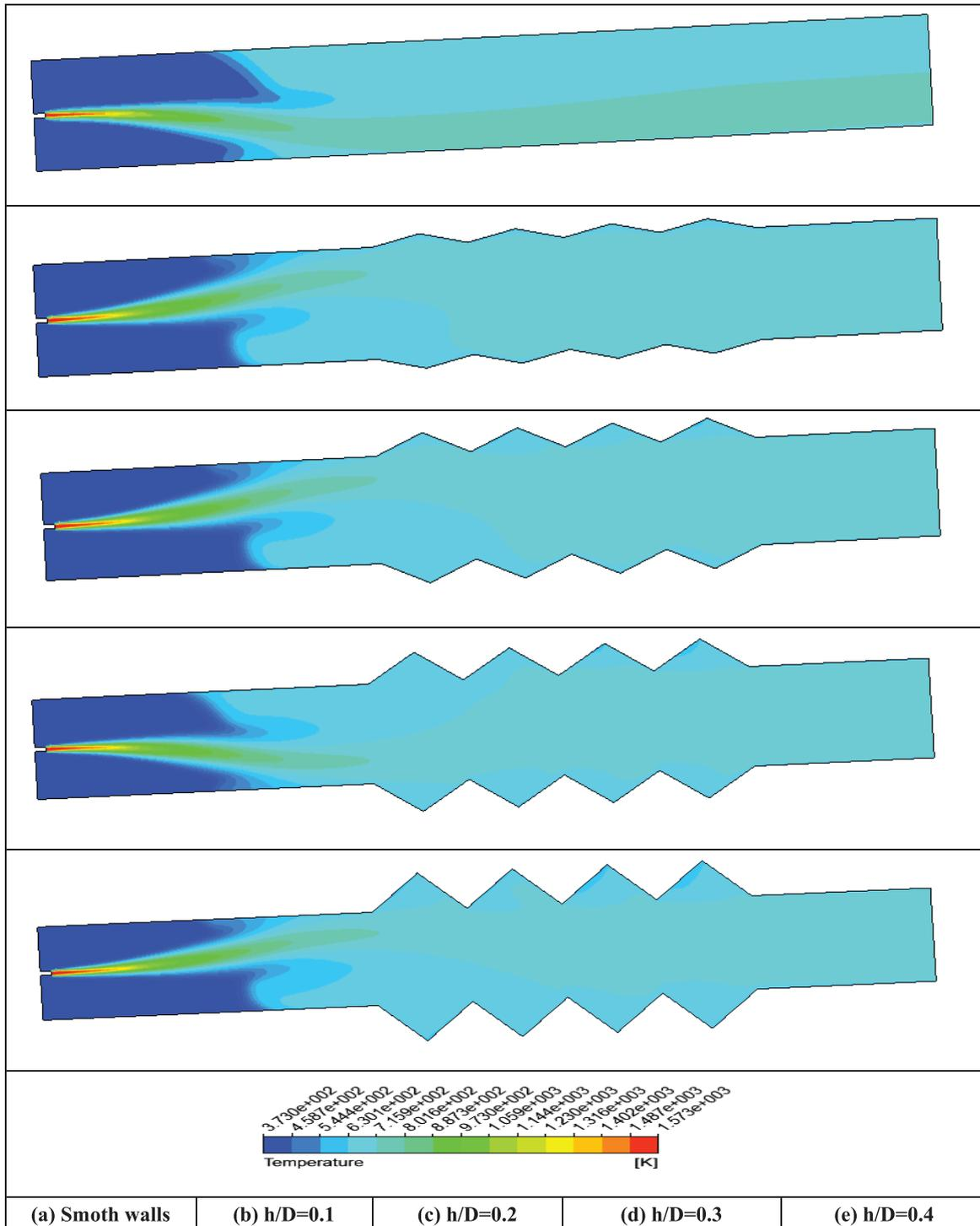
**Figure 11.** Isotherm contours of rotary kiln at different groove depths.
