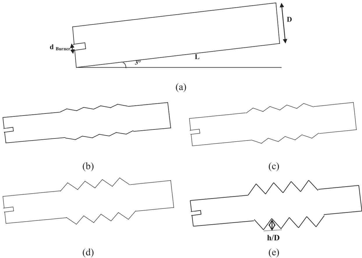
**Figure 3.** Two-dimensional model of rotary kiln: (a) Smooth walls, (b) grooved wall with  $h/D=0.1$ , (c) grooved wall with  $h/D=0.2$ , (d) grooved wall with  $h/D=0.3$ , (e) grooved wall with  $h/D=0.4$ .
