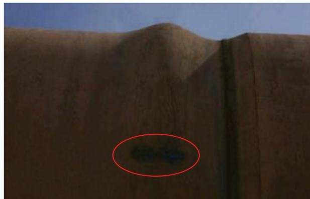
**Figure 2.** Deformation of the outer wall of the rotary cement kiln.
