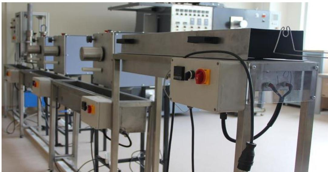
**Figure 2.** The pilot plant for wet spinning process
