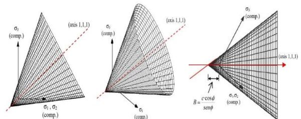
Fig. 5. Graphic representation of the DP criterion
