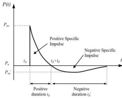
Fig. 2. Blast wave pressure – Time history (Abaqus 6.10)
