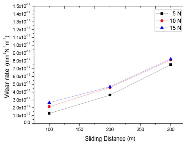
Fig. 6. Wear rate of Abrasive Samples
