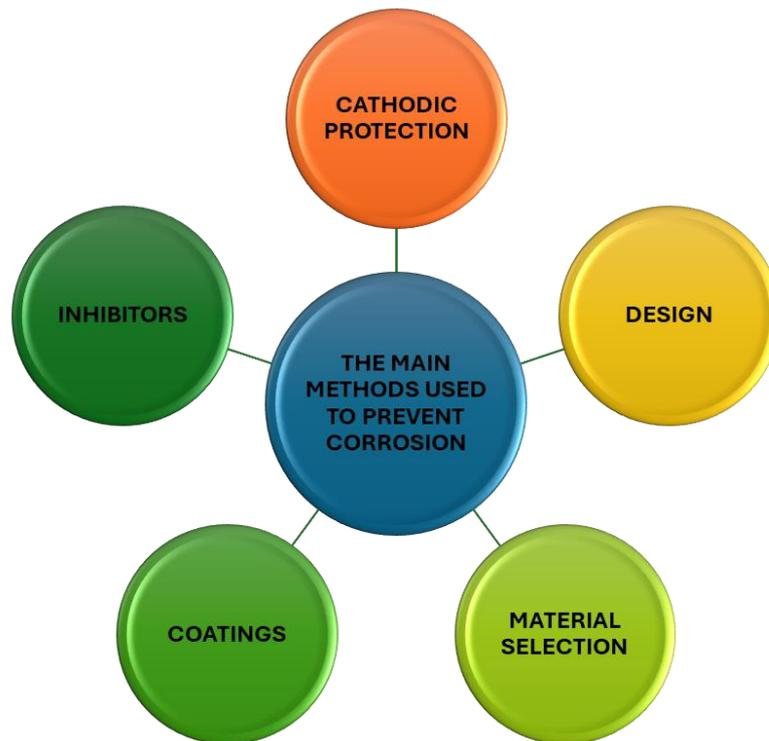
*Figure 1. The main methods used to prevent corrosion*
