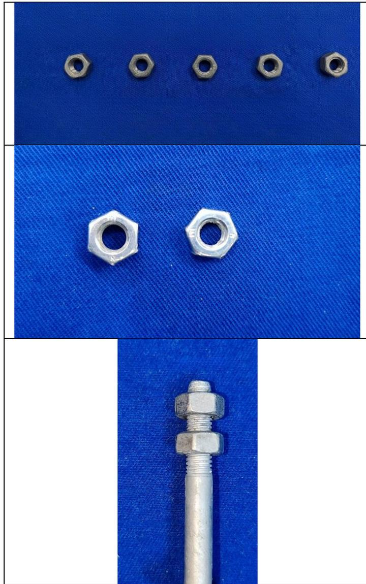
**Figure 3.** Visual inspection before the salt spray test
