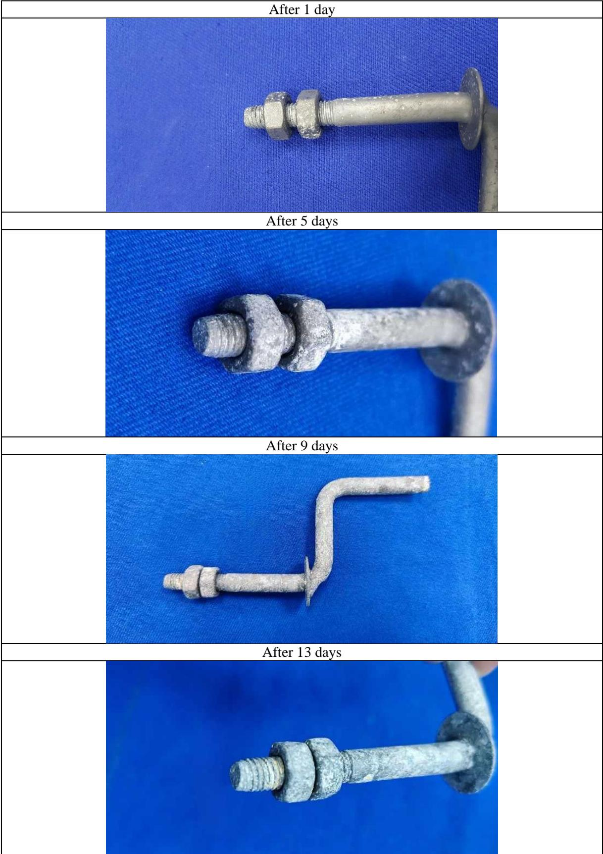
*Figure 4. Visual inspection after the salt spray test*
