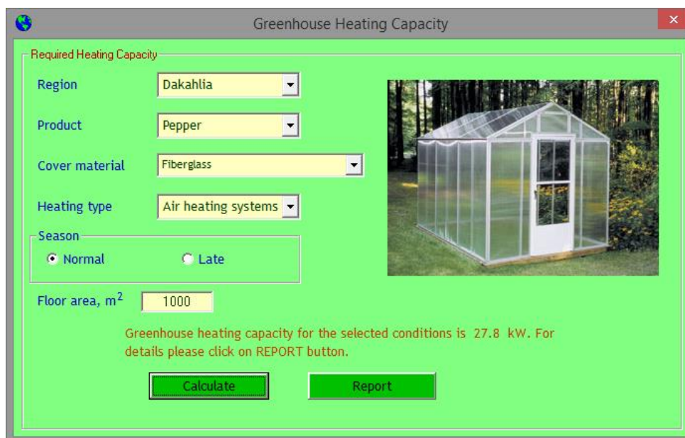
Figure 3. The calculation of the heating capacity needed for a pepper greenhouse established in the Dakahlia region
