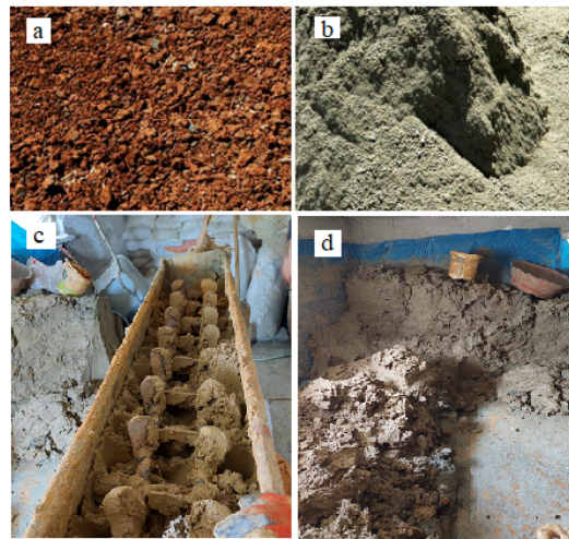
Figure 1: Clay and mud preparation a) red clay, b) oily clay, c) mud mixing device, d) prepared mud.
