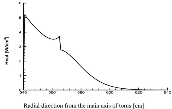
Figure 3. Heat generation profile for neutron load of  $4.2 \text{ MW/m}^2$  at outer first wall
