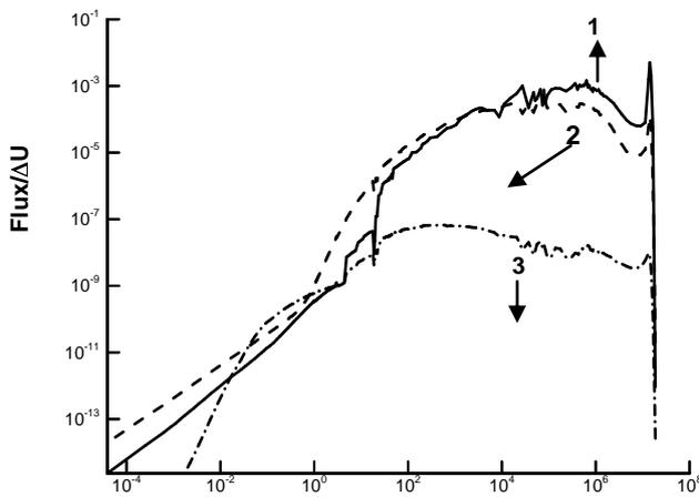
Figure 2. Neutron spectrums at different locations of the outer blanket
