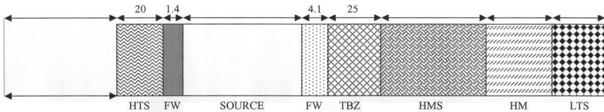
Figure 1. One-dimensional hybrid modeling of the ARIES-ST reactor
