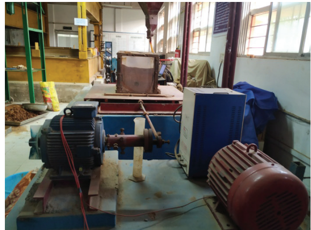
Figure 1. Shake table attached with Crank Shaft and slotted disc.
