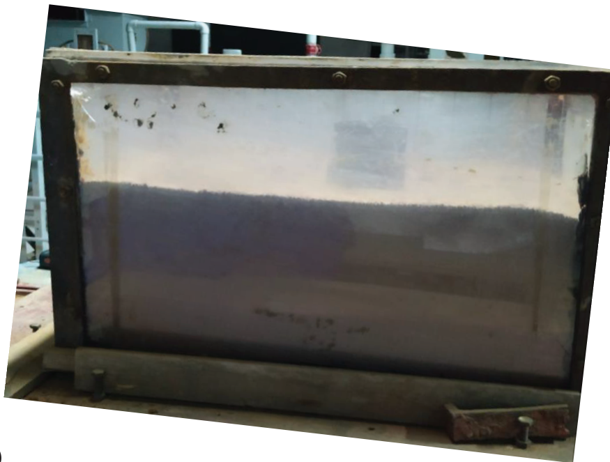
Figure 14. Failure mechanism observed immediately after the footing subjected 0.3g base shaking and 3Hz frequency.
