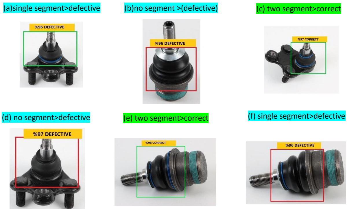
Figure 6. In the picture given in (a), the product is defective because it has a single segment; in (b), it is defective because it has no segment; in (c), it is correct. It has two segments: in (d), it is not very accurate because it has only a tiny segment; in (e), it has double segments. In (f), there are no rings at all. Therefore, it is a defective product.
