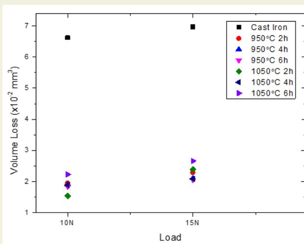
Figure 2. Wear volume loss measurement values
