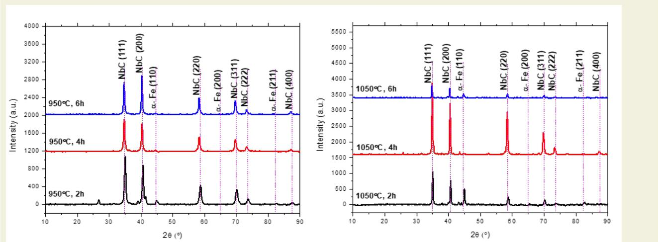
Figure 7. XRD analysis results of NbC-coated samples
