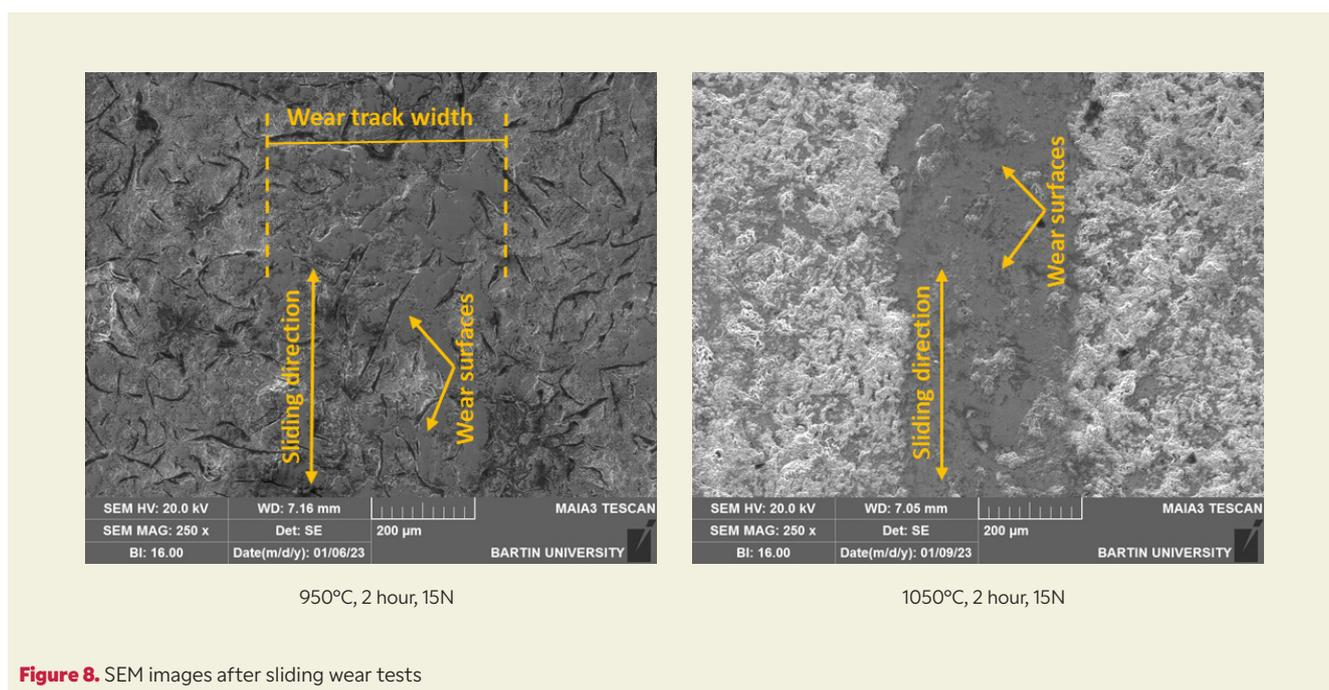
Figure 8. SEM images after sliding wear tests
