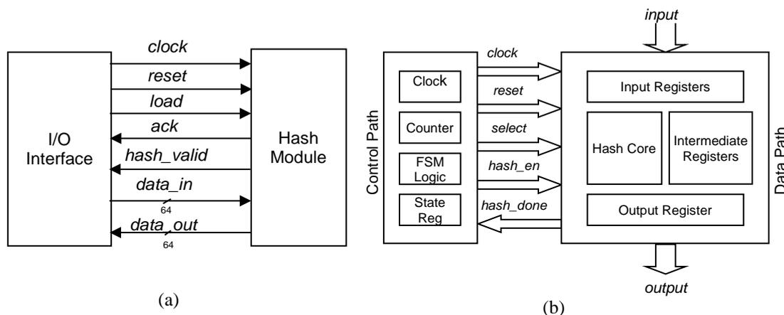
FIGURE 1. (a) Common I/O Interface (b) Hash Module separated in Control and Data paths
