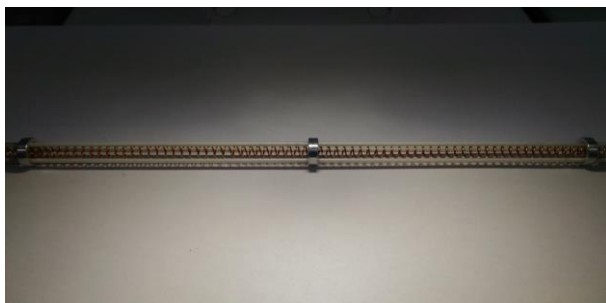
Fig. 4. Molybdenum helix coated with copper film.
