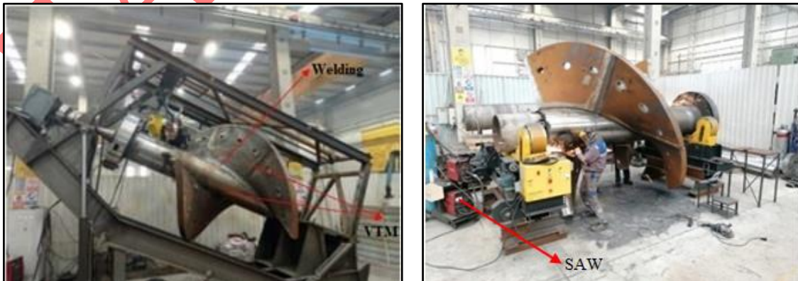
Figure 4. Welding process of spirals
