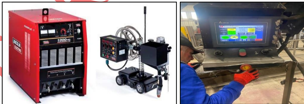
Figure 7. Designed submerged arc welding machine apparatus
