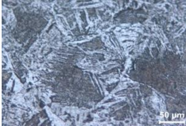
Figure 13. Upper region HAZ (Heat Affected Zone) A-A section
