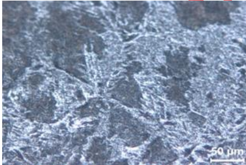
Figure 14. Lower zone HAZ (Heat Affected Zone) C-C section
