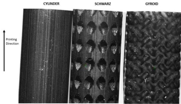
**Figure 8.** 3D printed TPMS based nerve guide conduits
