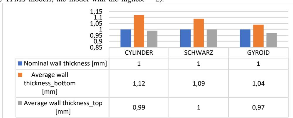
**Figure 16.** Average wall thickness measured from the bottom surface, average wall thickness measured from the top surface, nominal wall thickness measurements of all models
