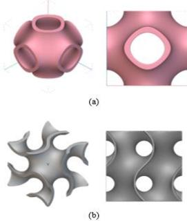
**Figure 4.** (a) Schwarz (b) Gyroid unit cells
