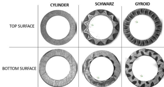
**Figure 15.** Bottom and top surface images of the produced nerve guide conduits
