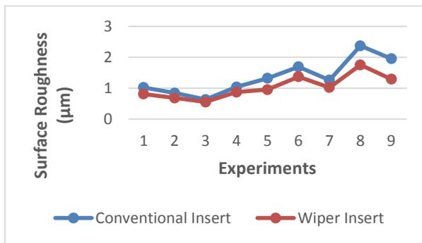
**Figure 3.** The surface roughness results
