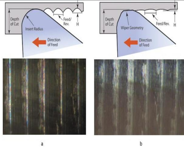
**Figure 4.** The surface roughness results for (a) conventional and (b) wiper insert
