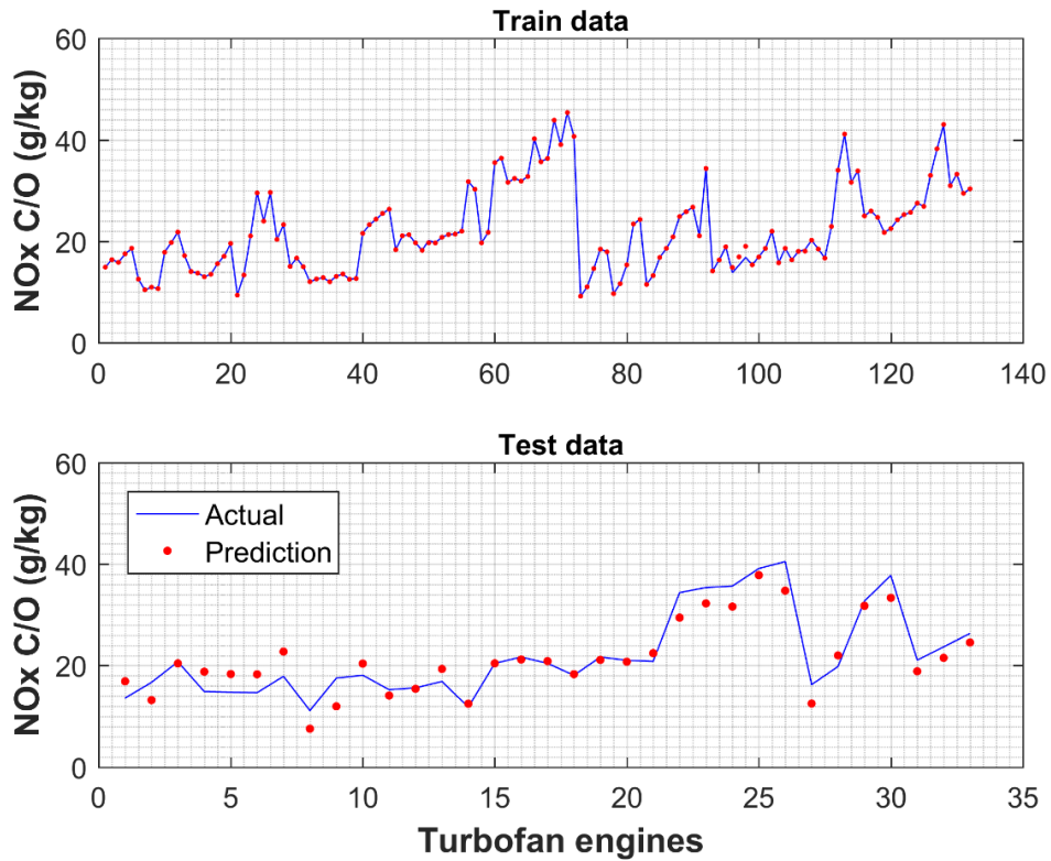
Figure 4. Comparison of actual NO x values and model values for the C/O phase
