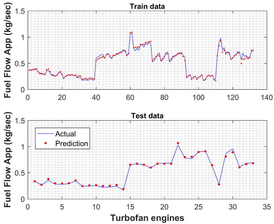
Figure 9. Comparison of actual FF values and model values for the app phase
