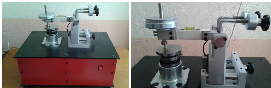
Figure 1. Schematic representation of the pin-on-disc test configuration.
