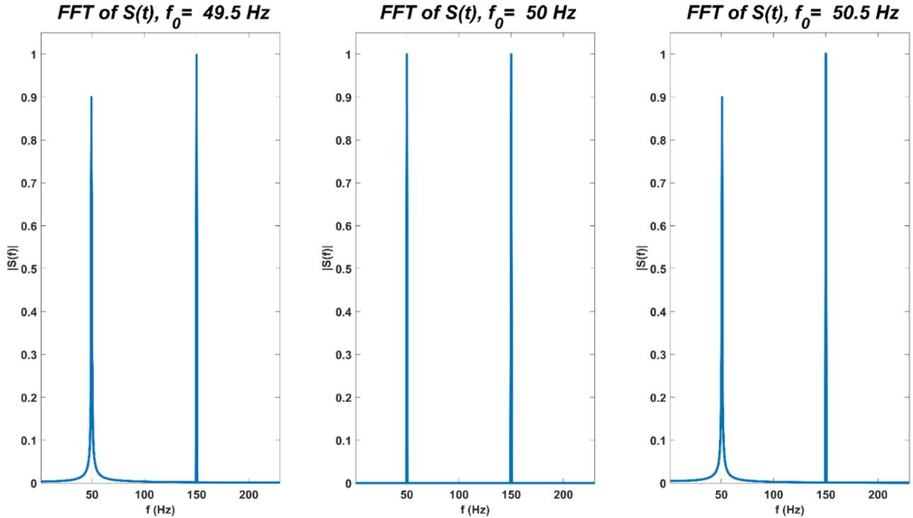
Figure 9. Effects of different main frequencies
