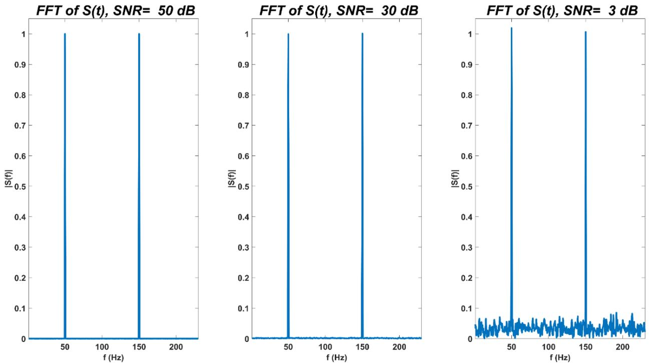
Figure 11. Effects of different SNR levels
