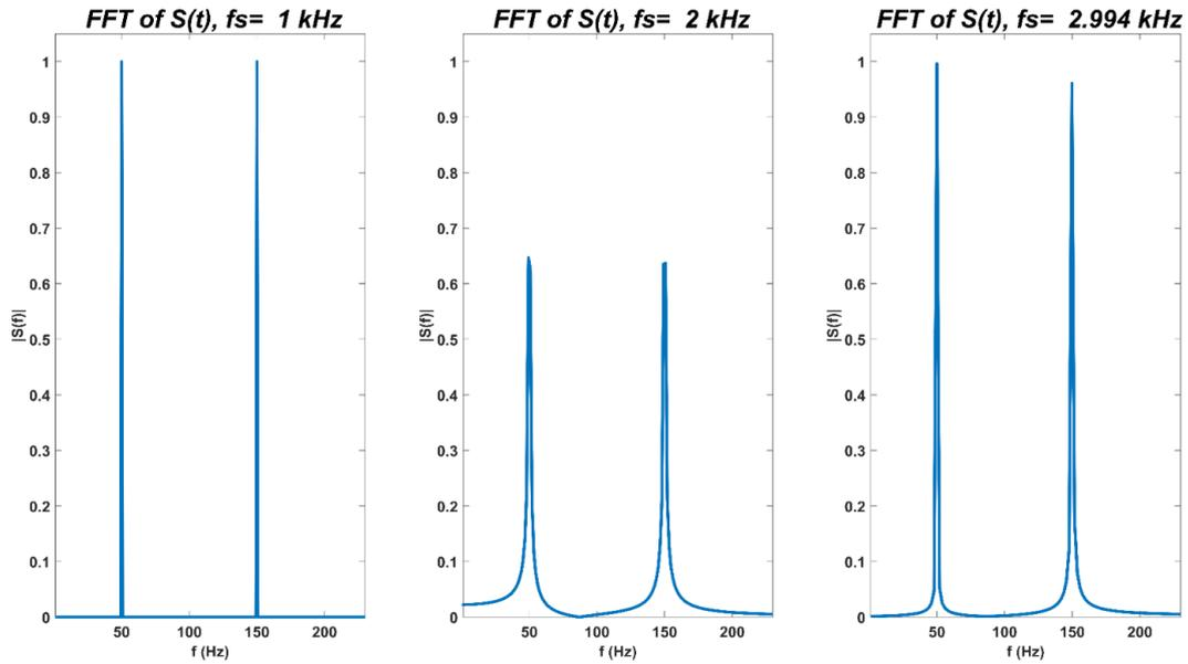
Figure 7. Effects of different sampling frequencies
