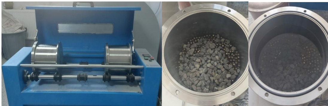
Figure 5. Micro-Deval Device, Micro-Deval drum, aggregate, steel shot and water mixture
