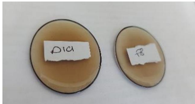
Figure 2. Fusing aggregates into glass tablets by fusion method
