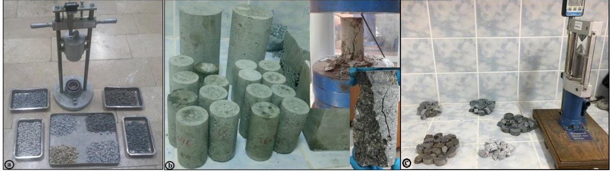
Şekil 2. Deneysel çalışmalar, ADDI deneyi (a), UCS örnekleri ve deneyi (b), PLI deneyleri (c) (Experimental studies, ADDI experiment (a), UCS samples and experiment (b), PLI experiments (c))
