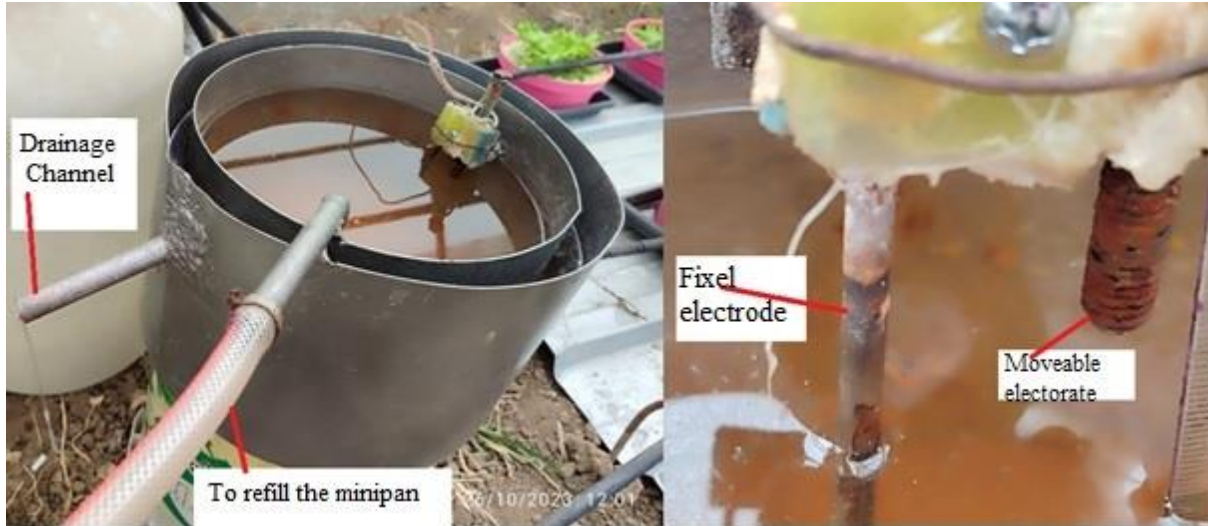
Figure 4. Mini evaporation pan and water level sensor (Yıldırım, 2016)
