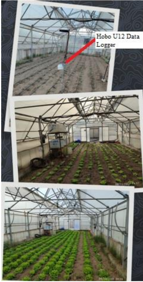
Figure 6. HOBO U12 data logger to save climatic data in the greenhouse.
