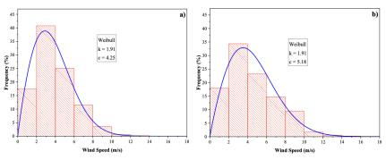
Figure 3: 2016 wind speed profile; a) 10m, b) 30m
