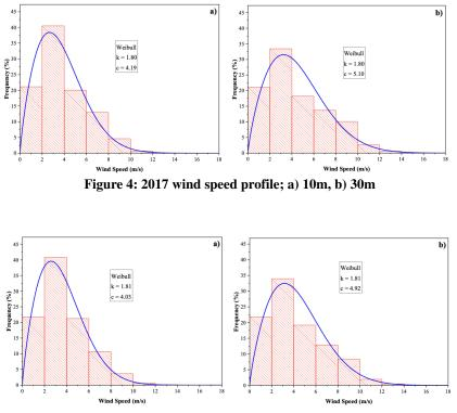
Figure 5: 2014 to 2017 wind speed profile; a) 10m, b) 30m
