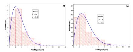
Figure 1: 2014 wind speed profile; a) 10m, b) 30m
