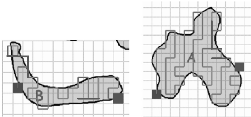
FIGURE 21. MGECA coverage solution for Zones A and B. Backtracked cells are shown with a red line.
