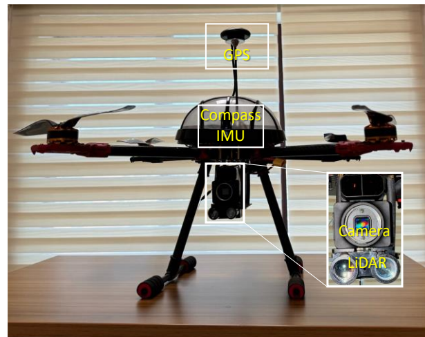
Figure 3. The comprehensive external representation of the autonomous UAV
