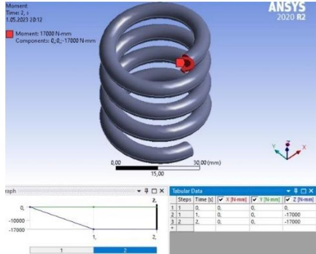
**Figure 4.** Initial torque applied and its steps.
