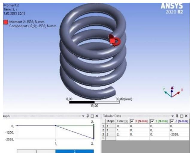
**Figure 5.** Second torque applied and its steps.
