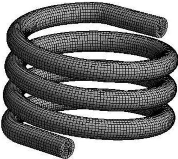
**Figure 3.** Finite element model of torsion spring [6].
