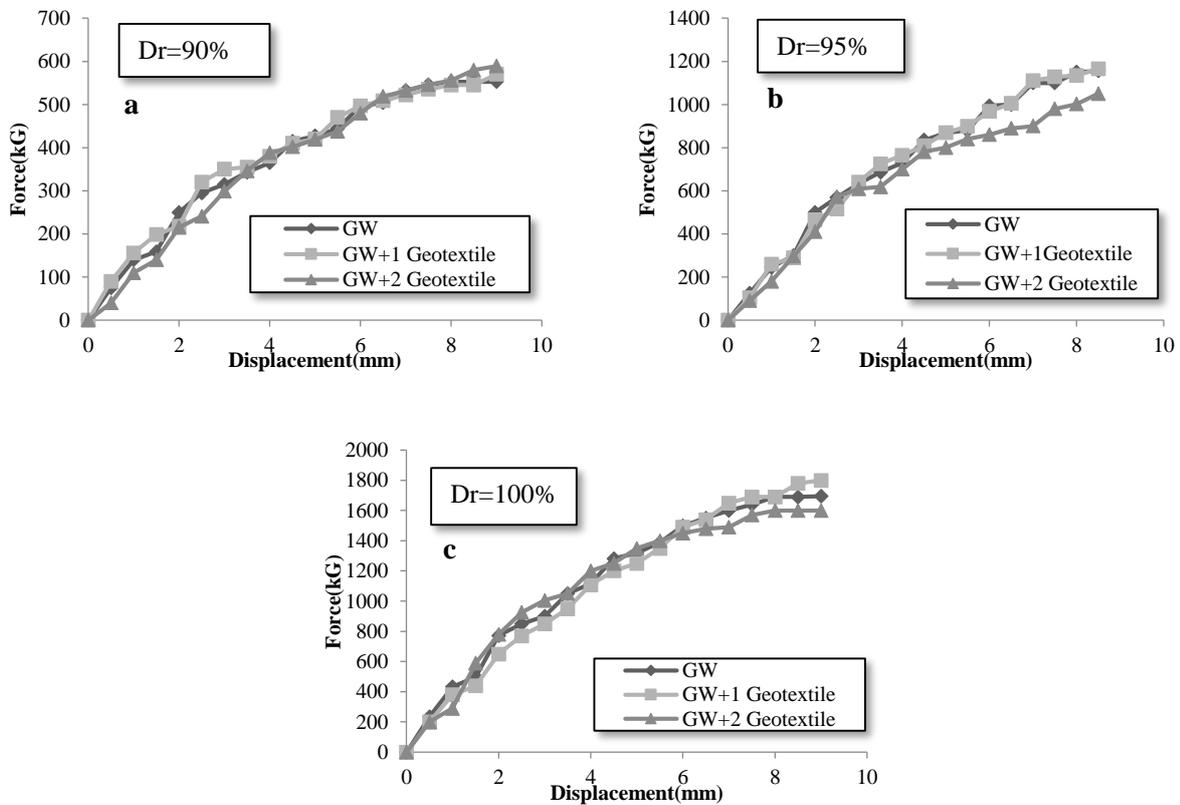
Figure 6. Comparison of gravel bearing capacity in reinforced and unreinforced position in several relative densities (Sadeghi azar et al., 2010)
