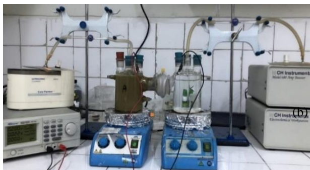
Figure 3. (a) Schematic representation (1/1': pH meter input, 2/2': electrode input, 3/3': gas outlet, 4/4': thermometer input) and (b) image of experiment system
