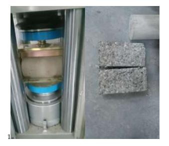
Figure 3. Split tensile test
