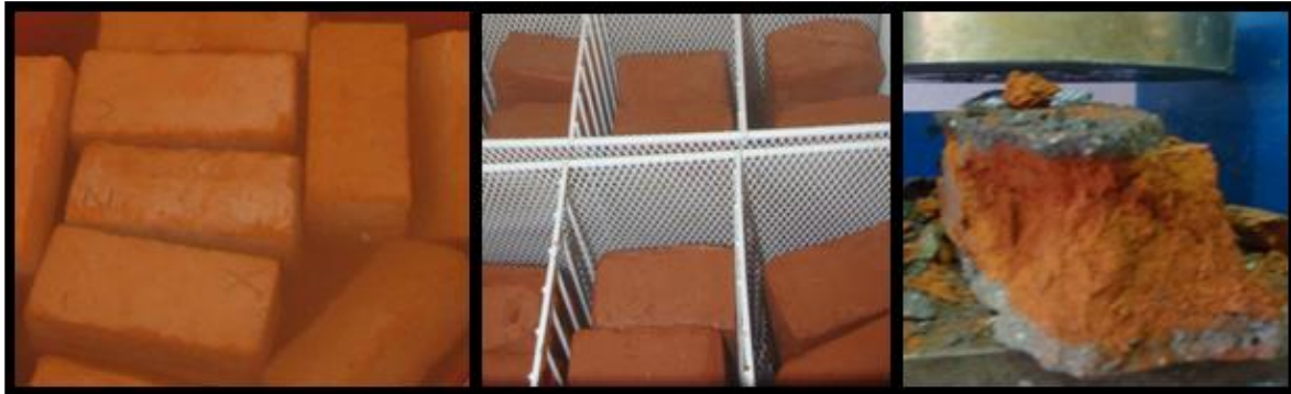
Figure 5. Handmade bricks with bottom ash and the tests
