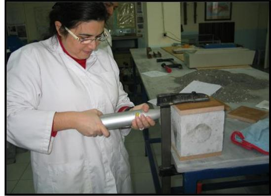
Figure 1. Application of a Schmidt Rebound Hammer (SRH).
