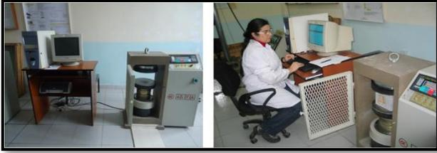
Figure 3. Compressive test equipment
