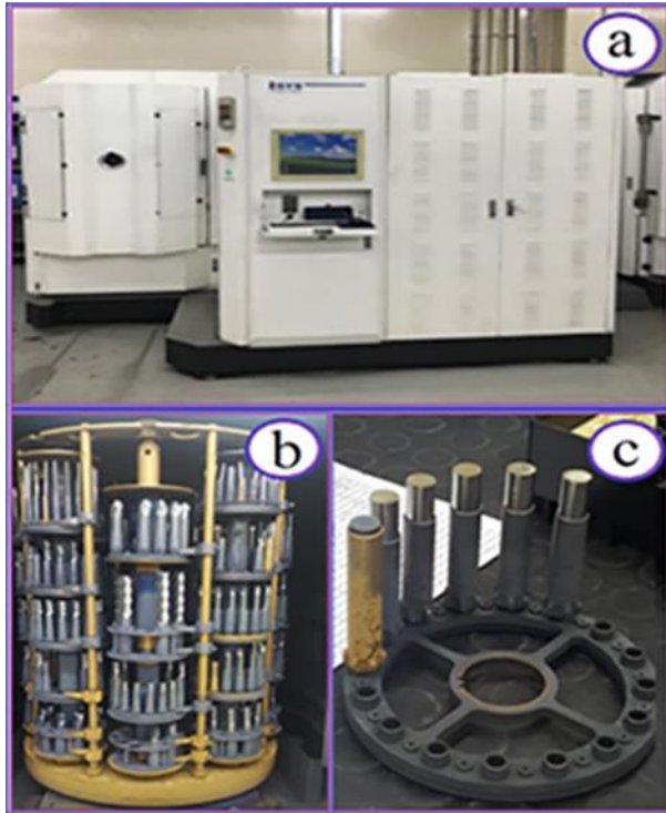
Figure 1 a) PVD coating machine (ISYS Intelligent System I 90A), b), c) The specimens were placed in the coating boxes
