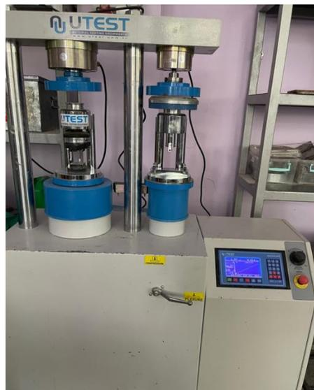
**Figure 5.** Three-point flexural test
