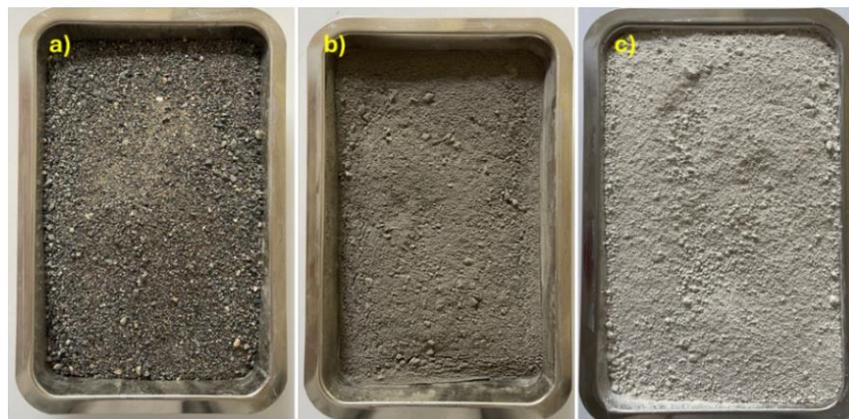
Figure 1. Dry ingredients used in mixes a) sand, b) PC, c) D
