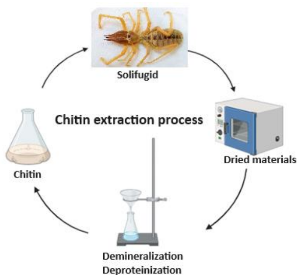
Figure 2. Scheme of chitin extraction process from Galeodes araneoides (Pallas, 1772)
