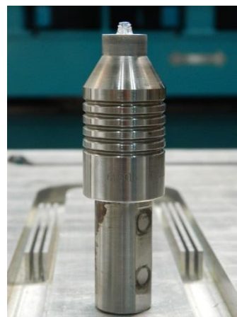
Figure 1. Photograph of FSW tool with threaded conical pin
